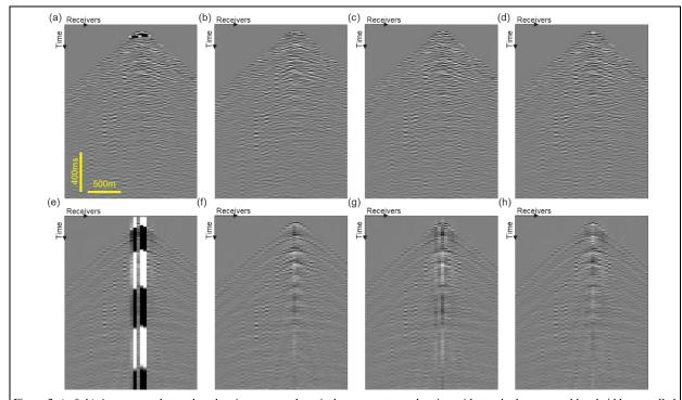
Figure 2: (a & b) A common-shot gather showing measured vertical component acceleration with standard source and bandwidth controlled source, respectively, c) precondition of a) with POCS and d) with PINNs. The bottom row (e-h) shows the corresponding images after integration into the particle velocity domain.
