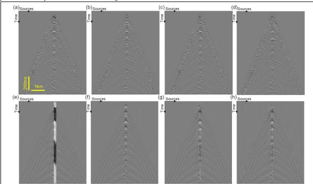
Figure 1: (a & b) A common-receiver gather showing measured vertical component acceleration with standard source and bandwidth controlled source, respectively, c) precondition of a) with POCS and d) with PINNs. The bottom row (e-h) shows the corresponding images after integration into the particle velocity domain.
