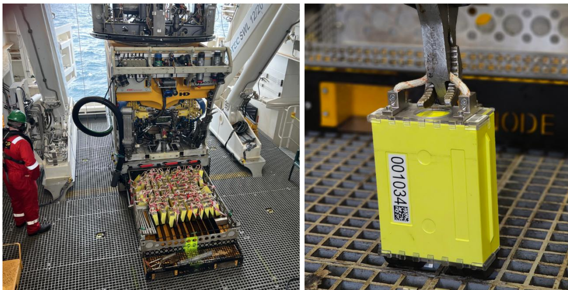
Figure 1 Portable and lightweight nodes (right) positioned in the skid (left) transported by the ROV for node deployment and retrieval.
